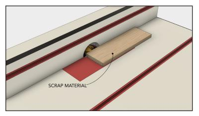
Run a piece of scrap material through the router and test the joint's fit. If the bit height and fence depth are correct, you're ready to route.
